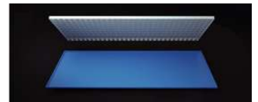
Mask is bonded to PCB revealing the COB chips through apertures in the mask
